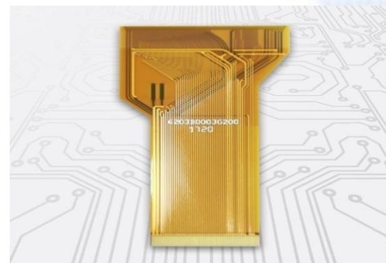
2 layers Precision circuit TP Module (VIA:0.1mm/ width&space:0.045)
