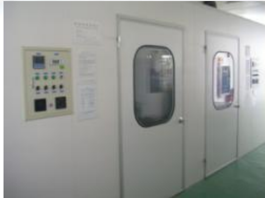
Burn-In Room 60°C
