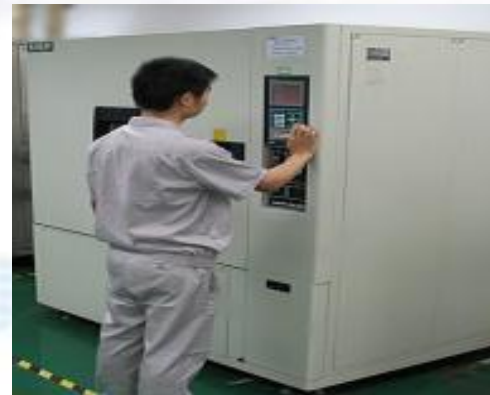
Thermal Cycle Chamber -40°C~150°C 0% ~ 99% RH
