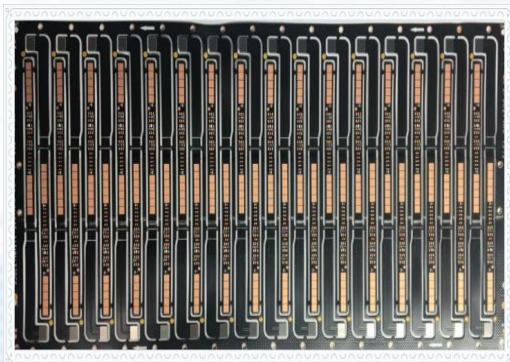
2 layers battery protection board
