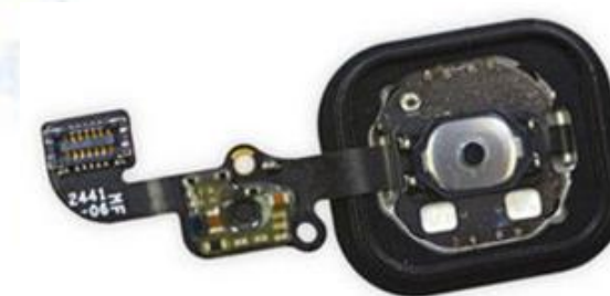
Rigid-Flex for Fingerprint identification module (FPCA)
