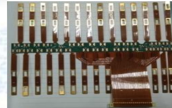
4 layers Rigid-Flex for High battery
