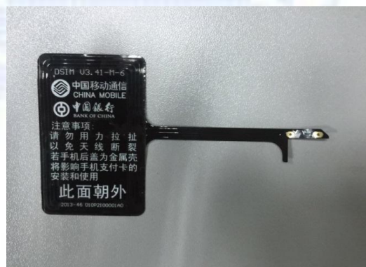
2 layers RFID / Antenna
